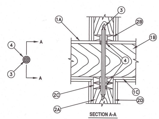
Floor-Ceiling Assembly — The 1 or 2 hr fire-rated solid or trussed lumber joist floor-ceiling assembly shall be constructed of the materials and in the manner specified in the individual L500 Series Floor-Ceiling Designs in the UL Fire Resistance Directory. The general construction features of the floor-ceiling assembly are summarized below:
