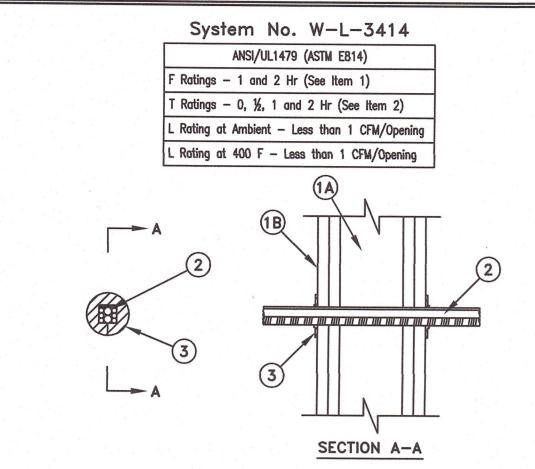
Wall Assembly — The 1 or 2 hr fire rated gypsum board/stud wall assembly shall be constructed of the materials and
